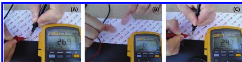
Figure 3. Mechanical adhesion test of the conductive AgNW–TiO 2 –PEDOT:PSS film. (A) Resistance measurement before tape peeling; (B) use adhesive tape to peel the film; (C) resistance measurement after tape peeling.
